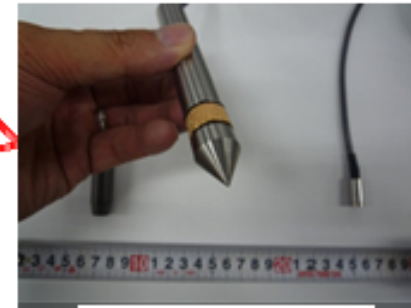
Pore pressure meter
