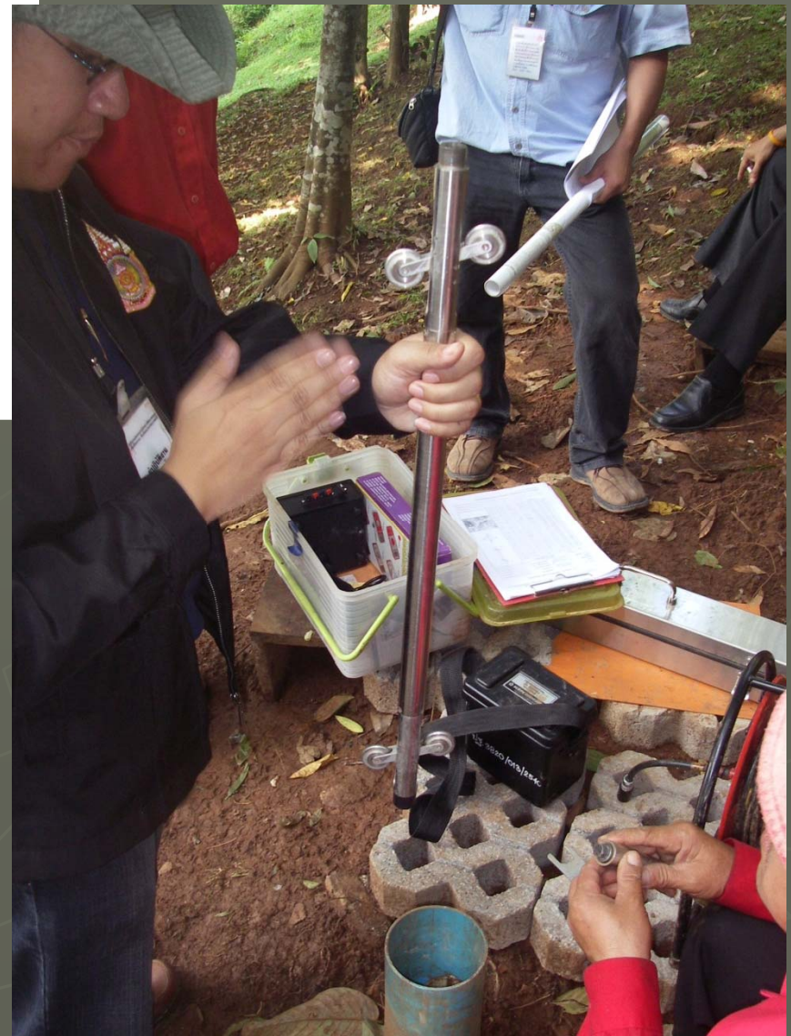
Inclinometer (torpedo type)
